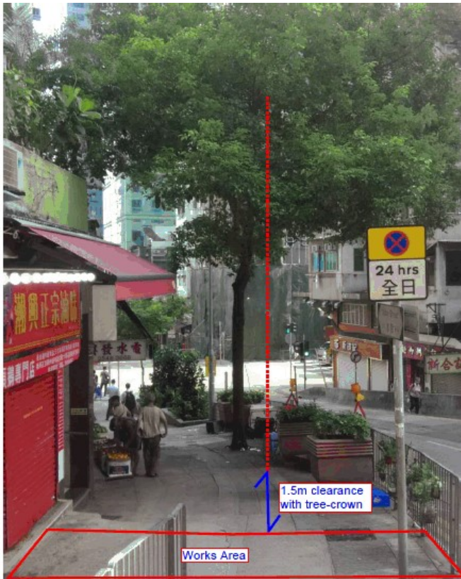
Photo 1: Vertical clearance between tree-crown and works area
